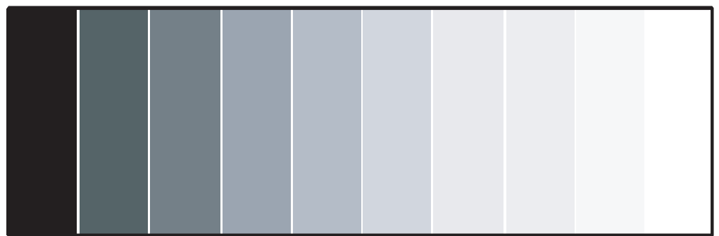
Figure 4-3. Typical Gray Bar Pattern for Adjusting Contrast
