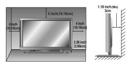
Table stand mount minimum allowable clearances for adequate ventilation.
