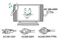
Use only the accessory cord designed for this product to prevent shock. The power supply voltage rating of this product is AC 100-240V, the power cord attached conforms to the following power supply voltage. Use only the power cord designated by our dealer to ensure Safety and EMC. When it is used by other power supply voltage, power cable must be changed. Consult your product dealer.
