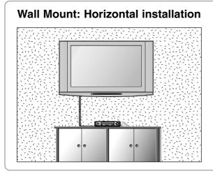
For proper ventilation, allow a clearance of 4" on each side and 2" from the wall. Detailed installation instructions are available from your dealer, see the optional Tilt Wall Mounting Bracket Installation and Setup Guide.
