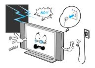
Unplug the monitor from the wall outlet and disconnect the antenna or cable system during a lightning storm or when left unattended and unused for long periods of time. This will prevent damage to the unit due to lightning and power-line surges.
