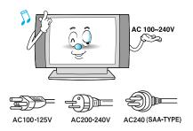
Use only the accessory cord designed for this product to prevent shock. The power supply voltage rating of this product is AC100-240V, the power cord attached conforms to the following power supply voltage. Use only the power cord designated by our dealer to ensure Safety and EMC.
