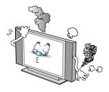
In case of smoke or strange smell from the monitor, switch it off, unplug it from the wall outlet and contact your dealer or service center
