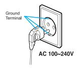
Use only a grounded or polarized outlet. For your safety, this monitor is equipped with a polarized alternating current line plug having one blade wider than the other. This plug will fit into the power outlet only one way. If you are unable to insert the plug fully into the outlet, try reversing the plug. If the plug still does not fit, contact your electrician to replace your outlet.
