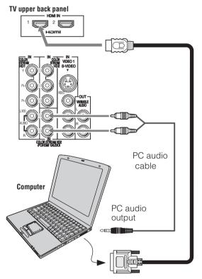
The HDMI input can accept and display VGA, SVGA, XGA, WXGA, SXGA, 480i (60Hz), 480p (60Hz), 720p (60Hz), 1080i (60Hz), and 1080p (24Hz/60Hz) signal formats. For detailed signal specifications, see page 61.
