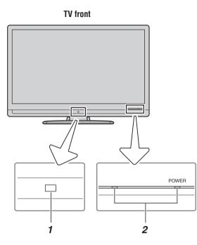
**1 Remote sensor** — Point the remote control toward this remote sensor.
