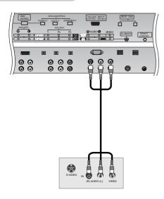
The TV has a special signal output capability which allows you to hook up a second TV or monitor.
