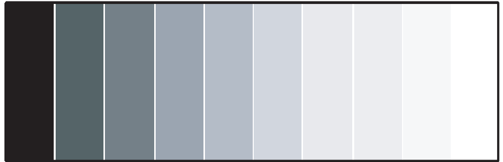
Figure 4-3. Typical Gray Bar Pattern for Adjusting Contrast
