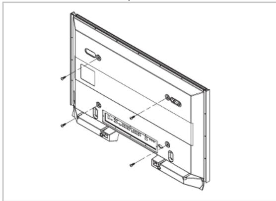
2. Insert screw B into the plastic hanger.
