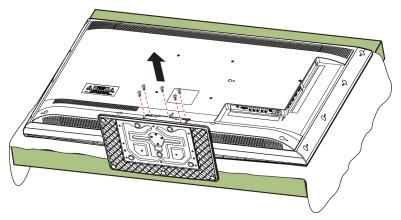
3 Attach the wall-mount bracket to your TV using the mounting holes on the back of your TV. See the instructions that came with the wall-mount bracket for information about how to correctly hang your TV.
