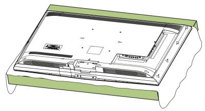
2 Secure the stand column to your TV with the five provided M4  $\times$  10 mm screws.
