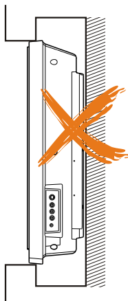
Air circulation is blocked
