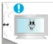
▶ Install your product in a well ventilated location. Ensure that there is a clearance of more than 10 cm from the wall.
