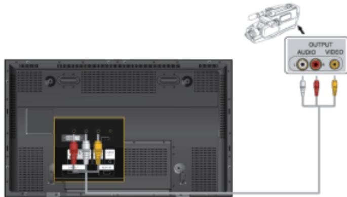
1. Locate the AV output jacks on the camcorder. They are usually found on the side or back of the camcorder. Connect a set of audio cables between the AUDIO OUTPUT jacks on the camcorder and the AV/COMPONENT AUDIO IN [L-AUDIO-R] on the PDP Display.
