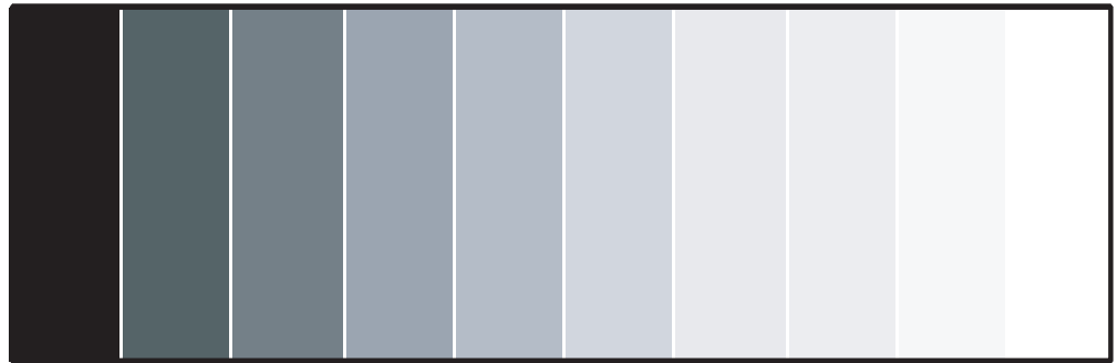
Figure 4-3. Typical Gray Bar Pattern for Adjusting Contrast
