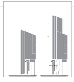
Auto stop: For your safety, the built-in automatic sensors will make the screen and loudspeaker stop if anything obstruct their movement. Remove the object and press • to continue switching the TV on or off.
