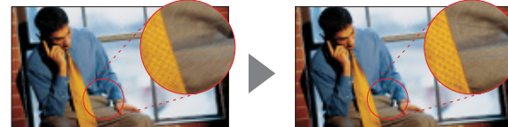
Previous Panasonic consumer LCD display product (simulation) (Noise is visible at diagonal edges.)
