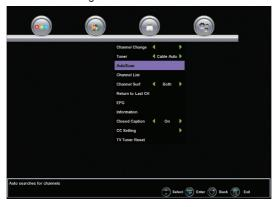
First Time connected to RF the system will automatically select the Autoscan function.
