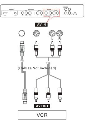
To watch a VCR image, select "AV" using SOURCE button on the remote control or front panel.
