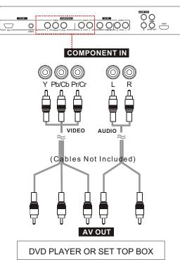
To watch a DVD or a broadcast from a set-top box using, the connection configuration shown above, press the SOURCE button on the remote control repeatedly to select COMPONENT as the input source.
