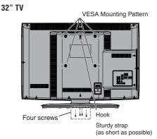
**CAUTION:** Always place the TV on the floor or a sturdy, level, stable surface that can support the weight of the unit. To secure the TV, use a sturdy strap from the hook(s) on the rear of the TV to a wall stud, pillar, or other immovable structure. Make sure the strap is tight, secure, and parallel to the floor.
