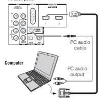
The HDMI input can accept and display VGA, SVGA, XGA, WXGA, SXGA, 480i (60Hz), 480p (60Hz), 720p (60Hz), 1080i (60Hz), and 1080p (24Hz/60Hz) signal formats. For detailed signal specifications, see page 56.
