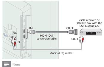
• Use an HDMI cable with the HDMI logo (a certified HDMI cable). High Speed HDMI cable is recommended for the better compatibility.
