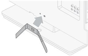
2 Pass cables through the cable management tie to avoid tangles.
