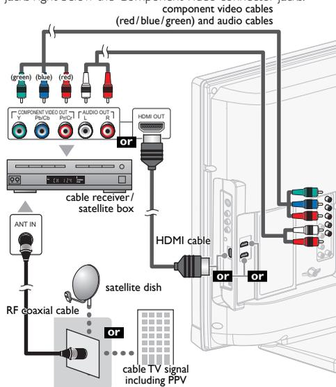
You can also connect this unit to the cable receiver or satellite box other than the HDMI or the Component Video output jacks or Composite Video output jack (► p.25, 26) because they might have different output jacks.
