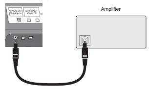
1) Connect the optical cable from underneath the television to the back of the amplifier.
