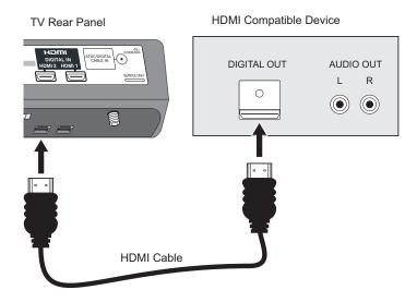
Connect the HDMI Cable from the DIGITAL OUT on the back of your DTV or HDMI device, to the DIGITAL-IN on the back of your television.
