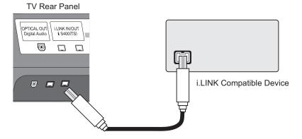
Connect the i.LINK cable from underneath the TV to the back of the i.LINK compatible device.
