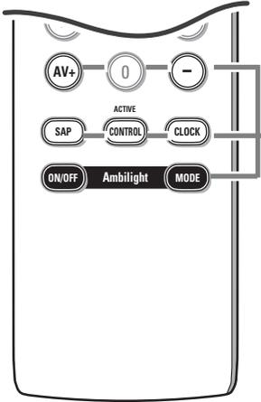
**AV+** Keep this button pressed and then press repeatedly to select **AV1, AV2, HDMI (AV3), SIDE** or **TV channels** when in TV mode, according to where you connected the accessory devices (p. 19).
