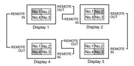
\* With the 3×3 video wall, connect the final display to the first display the same way as with 2×2 video wall.
