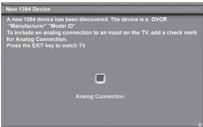
Figure 5. The ClearThought Auto Input sensing screen for IEEE 1394 devices. Place a check in the Analog Connection box if your device has both analog and digital outputs.
