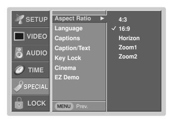
Lets you choose the way that an analog picture with a 4:3 aspect ratio is displayed on your TV 16:9 aspect ratio TV screen. When you receive an analog picture with a 4:3 aspect ratio on your 16:9 TV, you need to specify how the picture is to be displayed according to your preference.
