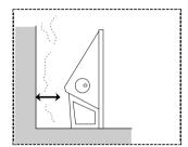
Make sure to put the product at a distance (of about 10cm/4inch) from the wall so that adquate ventilation can be provided.
