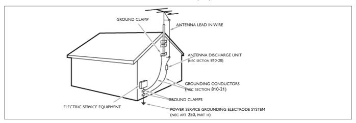
Note to the CATV system installer: this reminder is provided to call the CATV system installer's attention to Article 820-40 of the NEC that provides guidelines for proper grounding and, in particular, specifies that the cable ground shall be connected to the grounding system of the building, as close to the point of cable entry as practical.
