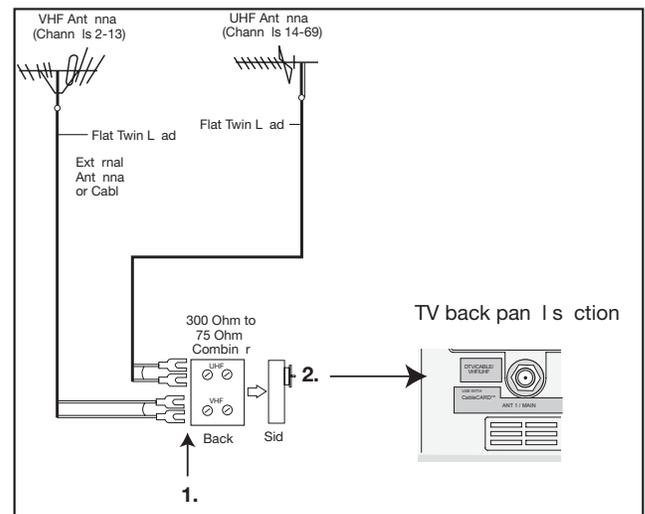
Figure 4. Connecting separate UHF and VHF Antennas
