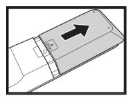
2 Insert the batteries paying attention to the polarity markings inside the battery compartment.
