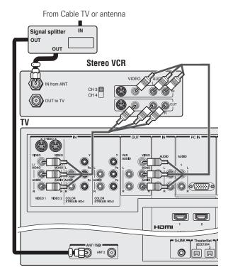
**Note:** The VIDEO/AUDIO OUT terminals output signals from the ANT 1, ANT 2, VIDEO 1, VIDEO 2, and VIDEO 3 terminals when the applicable input mode is selected.
