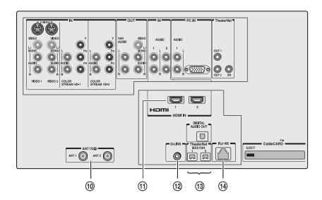
① ANT-1 (CABLE) IN and ANT-2 IN — Two inputs that support analog (NTSC) and digital (ATSC) off-air antenna signals and analog and digital (QAM) Cable TV signals.
