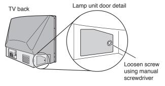
4. Using a manual screwdriver, loosen the two screws on the lamp
