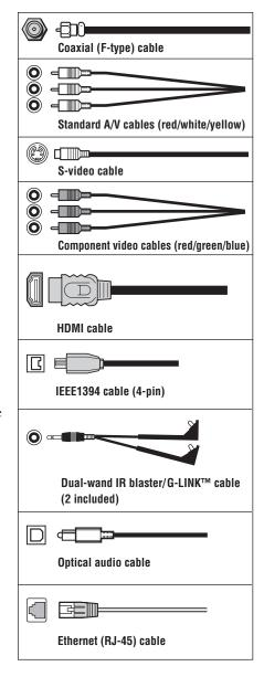
Note: Although your TV includes both HDMI and IEEE1394 connections, it may not operate with another device you have that includes such a connection. For example, the IEEE1394 ports are not intended to operate with current model Mini DV camcorders, and the HDMI input is not intended for connection to a computer. Copyright protection requirements may also prohibit or limit connectivity. See page 21 for details about the HDMI input. See pages 25–27 for details about the IEEE1394 ports.
