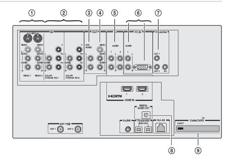
① VIDEO 1 IN and VIDEO 2 IN — Two sets of standard (composite) video and standard audio inputs plus optional S-video inputs for connecting devices with composite video or S-video output.
