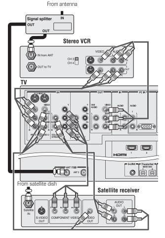
**Note:** The VIDEO/AUDIO OUT terminals output signals from the ANT 1, ANT 2, VIDEO 1, VIDEO 2, and VIDEO 3 terminals when the appropriate input mode is selected.
