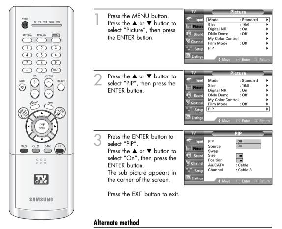
$\ensuremath{\mathsf{Press}}$  the PIP button on the remote control repeatedly to activate or deactivate the PIP.
