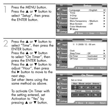
You can set the hour, minute, channel, and volume directly by pressing the number buttons on the remote control.
