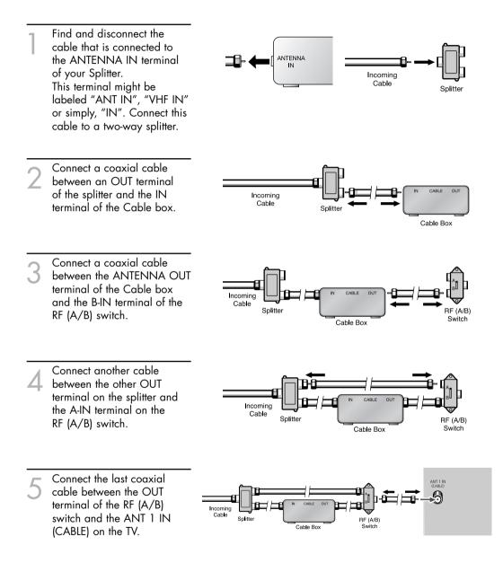
After you've made this connection, set the A/B switch to the "A" position for normal viewing. Set the A/B switch to the "B" position to view scrambled channels. (When you set the A/B switch to "B", you will need to tune your Set-Top Box to the Cable box's output channel, which is usually channel 3 or 4.)
