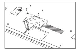
2 Mount the base to the stand with the provided three (3) flat head screws
