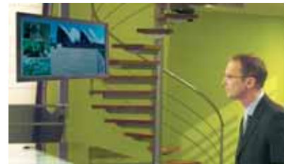
Wrong color balance results in a bluish image in backdrop applications
