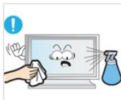
▶ When cleaning the product, do not spray water directly onto the main body of the product.
