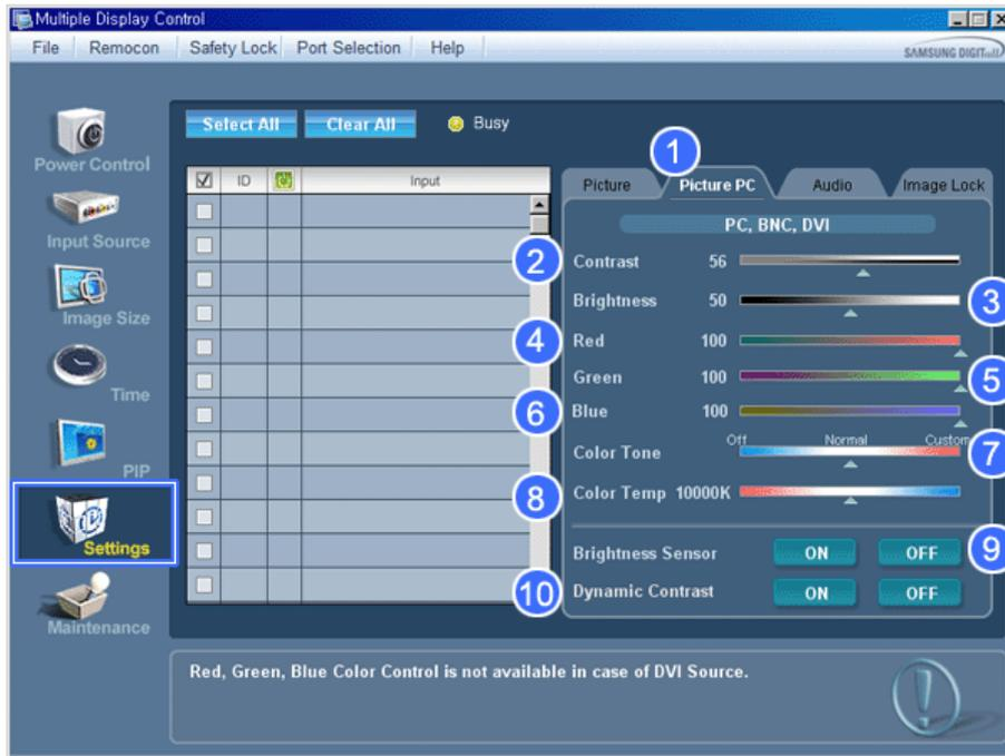
\* Info Grid shows some basic information necessary to Settings Control. When each function is selected, the set value of the selected function is displayed in the slide. When selected, each function fetches the value for the set and displays it on the slide bar. When "Select All" is chosen, the default value is displayed. Changing a value in this screen will automatically change the mode to "CUSTOM."
