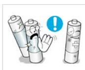
▶ Use only the specified standardized batteries, and do not use a new battery and a used battery at the same time.
