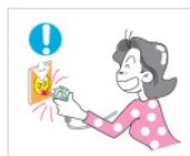
▶ To disconnect the apparatus from the mains, the plug must be pulled out from the mains socket, therefore the mains plug shall be readily operable.
