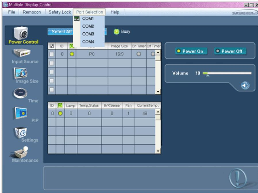
1. The Multiple Display Control is originally set to COM1.
