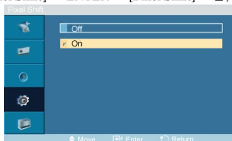
To prevent after-images on the screen you can use this function, so that every minute pixels on the LCD are moved in horizontal or vertical direction.
