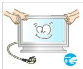
▶ When moving the product, turn the power off and disconnect the power plug, antenna cable, and all the cables connected to the product.
