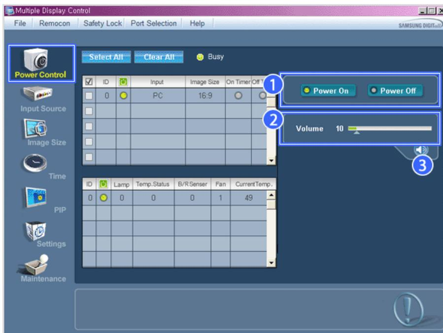
\* Power Control allows controlling some of the functions of the selected display.
