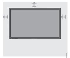
Regardless of whether you place BeoVision 4 on a table stand or in a wall bracket, make sure to leave adequate space around the screen for ventilation purposes, as described to the right.
