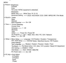
During menu operation the bottom of the on screen display will show which controls can be used for menu navigation.
