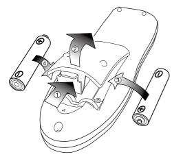
Install two "AA" 1.5 volt batteries so that the "+" and "-" marks on the batteries match the "+" and "-" marks inside the unit into the remote control handset.
