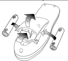
Install two "AA" 1.5 volt batteries so that the "+" and "-" marks on the batteries match the "+" and "-" marks inside the unit into the remote control handset.
