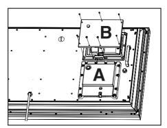
DO NOT REMOVE SILICA GEL SACHETS FROM INSIDE LD-NET TERMINAL COVER (B) AND TERMINAL COVER (A).
