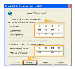
In step 2 of MagicInfo Setup Wizard, you don't have to go to Network Setting on the desktop to make your settings for TCP/IP. You just do that at step 2 of MagicInfo installation.
