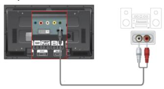
1. Connect a set of audio cables between the AUX L, R jacks on the AUDIO SYSTEM and AUDIO OUT on LCD Display.
