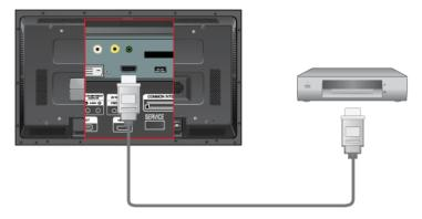
Connect input devices such as a Blu-Ray/DVD player to the HDMI IN terminal of the LCD Display using an HDMI cable.
