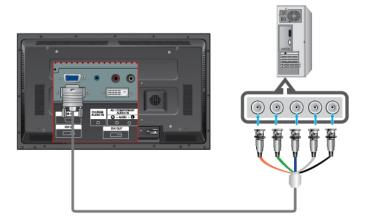
1. Connect the RGB/COMPONENT IN port on the monitor to the BNC port on the PC using the D-SUB to BNC cable.
