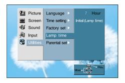
\*\*Do not reset the "Lamp Time" without exchanging the lamp with a new one.
