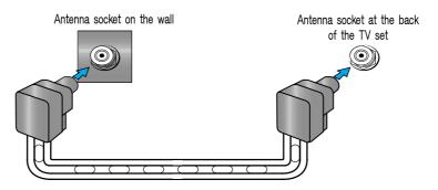
Feeder cable connection with the aombining adapter
