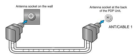
Feeder cable connection with the combining adapter
