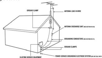
Remember, the screen of the coaxial cable is intended to be connected to earth in the building installation.
