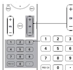
Press **CHANNEL +/-** on the side of the TV. For digital channels, press a number (1 to 135) followed by a dot “.” and then the corresponding sub channel number (1 to 135). e.g. 108.30.
