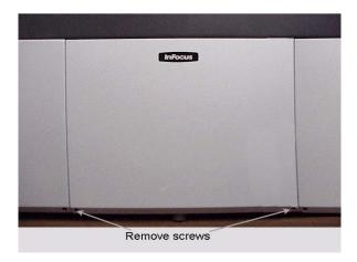
To access the adjustments on the small mirror, remove two screws under the center access panel and remove the panel.
