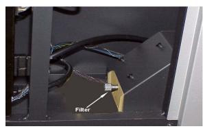
Filter housing showing captive fastener on filter.
