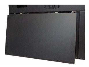
2. Remove the left access panel by removing the two 6x32 screws at the bottom of the panel and sliding the panel to the left.
