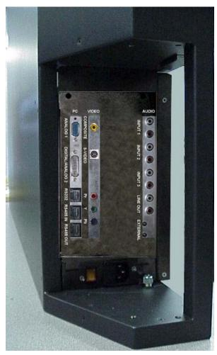
TD61 Signal Input Panel, Left Side View
