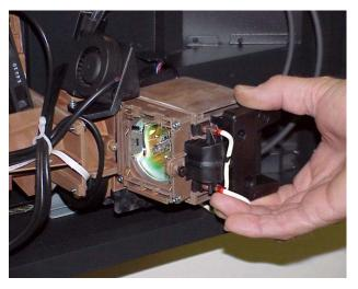
5. Remove the defective lamp.
