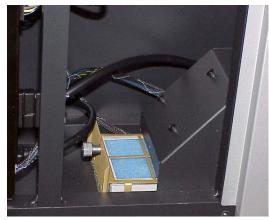
3. Remove filter from filter housing.
