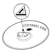
4 Secure the bottom plate with the four provided silver screws
