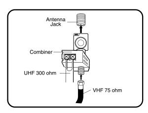
Connect the VHF 75 ohm cable and UHF 300 ohm twin-lead wire to the Combiner (not supplied).
