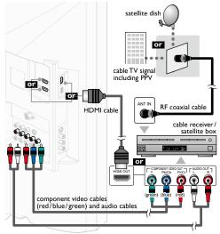
You can also connect this unit to the cable receiver or satellite box other than the HDMI or the Component Video output jacks or Composite Video output jack (**\*\*\* p.26**) because they might have different output jacks.
