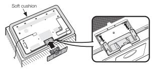
4 Insert and tighten the 4 screws into the 4 holes on the rear of the stand unit.
