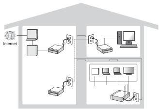
Up to four devices can be connected to the HN-VA400U adapter.
