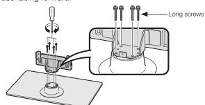
3 Insert the stand into the openings on the rear of the TV.
