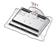
Remove the screws and detach the stand from the TV.
