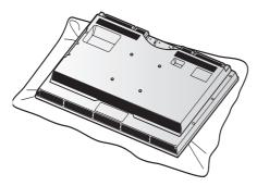
Assemble the TV and install the 6 screws into the holes as shown.
