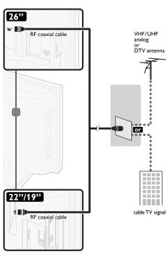
Once connections are completed, turn on the unit and begin initial setup. Channel scanning is necessary for the unit to memorize all available channels in your area. [Initial Setup] IIII p.15
