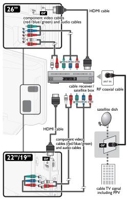
Required cables and connecting methods of the cable receiver/ satellite box, or the availability channel for the clear QAM may differ depending on the cable/satellite provider or local TV broadcaster.
