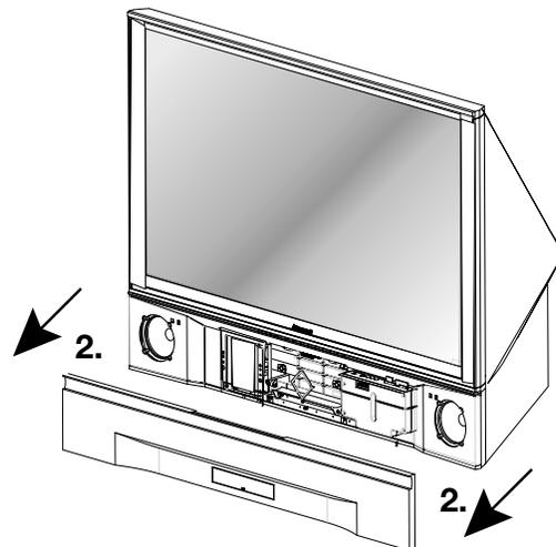
4. Remove the plastic cover and set aside with the screws.
