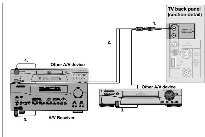
Figure 17. Connecting IR Emitter NetCommand
