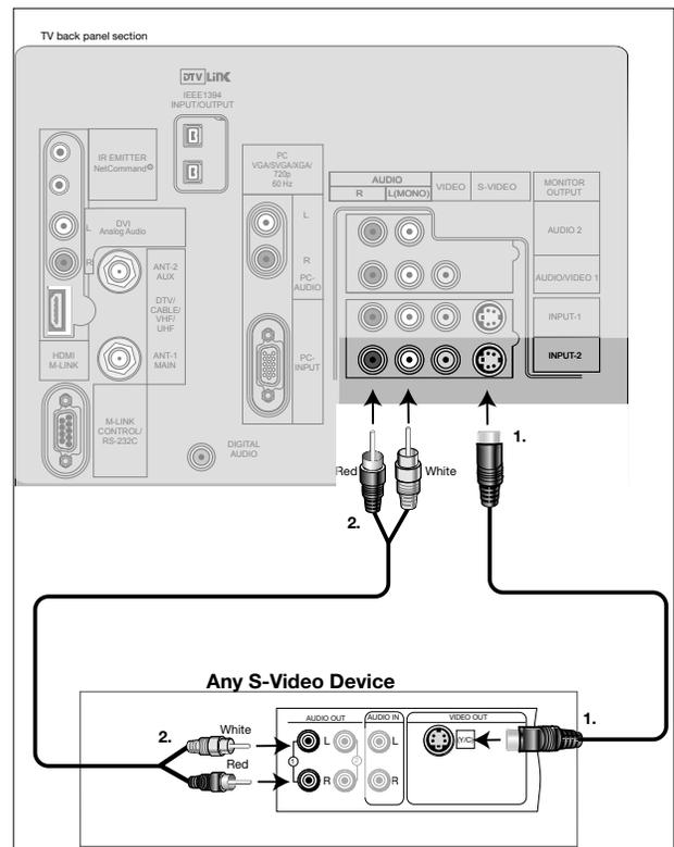
Figure 8. Connecting a Satellite Receiver with S-Video
