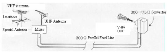
• When using a  $300\Omega$  parallel feed line, it must be connected to a  $300\Omega$  to  $75\Omega$  converter and then connected to the VHF/UHF terminal of the tuner.
