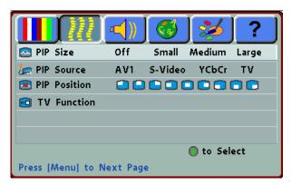
Press the ▲/▼ keys to enter the Quick Menu to select TV for the PIP Source (when OSD is not being displayed)
