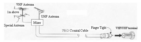
• When using a  $75\Omega$  Coaxial Cable, it can be connected directly to the VHF/UHF terminal of the tuner.
