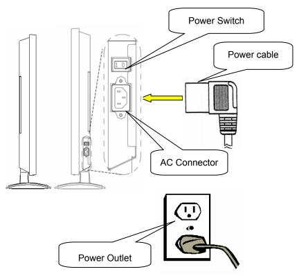
Connect the power cable female end to the display, and then connect the male plug to the wall outlet.
