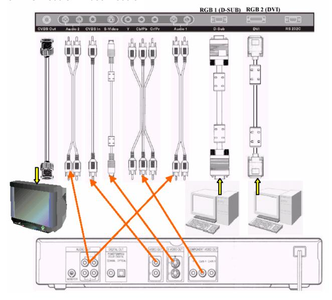
The functions of D-Sub, DVI and RS-232 terminals are the same as for the PC module.
