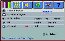
Press the ▼ key to highlight Channel Program and press the ► key to commence Channel Scan.
