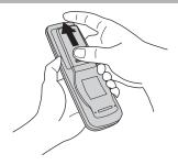
(1) To remove the cover, slide it outwards while pressing it down.
