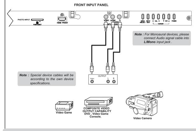
NOTE: 1. Completely insert connection cord plugs when connecting to front panel jacks. If you do not, the played back picture may be abnormal.
