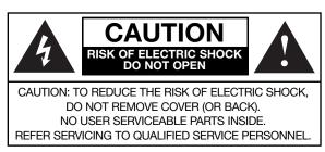
The lightning flash with arrowhead symbol, within an equilateral triangle, is intended to alert the user to the presence of uninsulated "dangerous voltage" within the product's enclosure that may be of a sufficient magnitude to constitute a risk of electric shock to a person.
