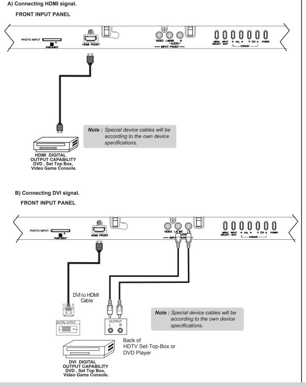
NOTE: 1. Completely insert connection cord plugs when connecting to front panel jacks. If you do not, the played back picture may be abnormal.
